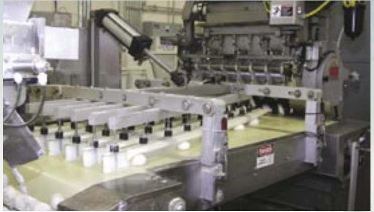
▲ The 6-pocket divider eliminates the need to turn pans and offers the bakery additional volume capacity.
