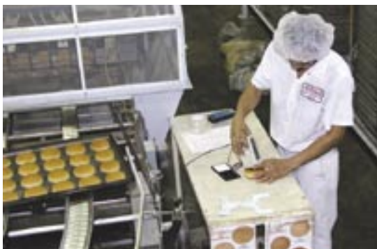
▼ Orlando Melendez, production, Q.A. manager, performs color meter, height and width measurement, and seed coverage tests prior to depanning baked buns.
