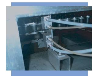
The Automatic Lubrication Package showed a 75% reduction of oil usage vs. previous technology, less energy was required to drive the system.
