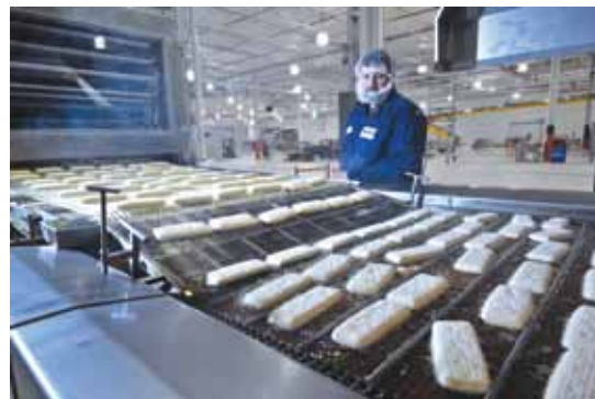
Maintenance employee Shawn Whitmore looks on as proofed long johns enter the 28-ft-long fryer, where they will cook for 97 seconds.
