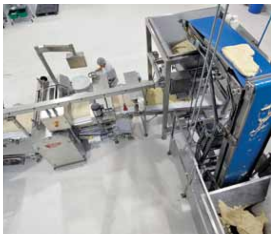
Chunked dough pieces travel up the twin-belt dough elevator to a horizontal conveyor that delivers them to the dough former.
