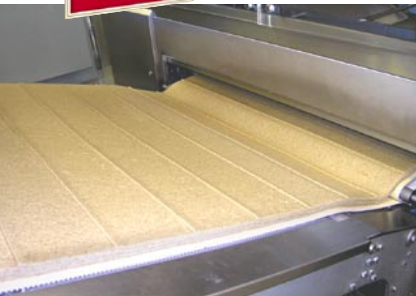
◀▲ Seven-layer lamination for whole-wheat cracker dough begins the sandwich cracker process, while Paula Cantin and Denis Leclerc monitor downstream oven settings.
