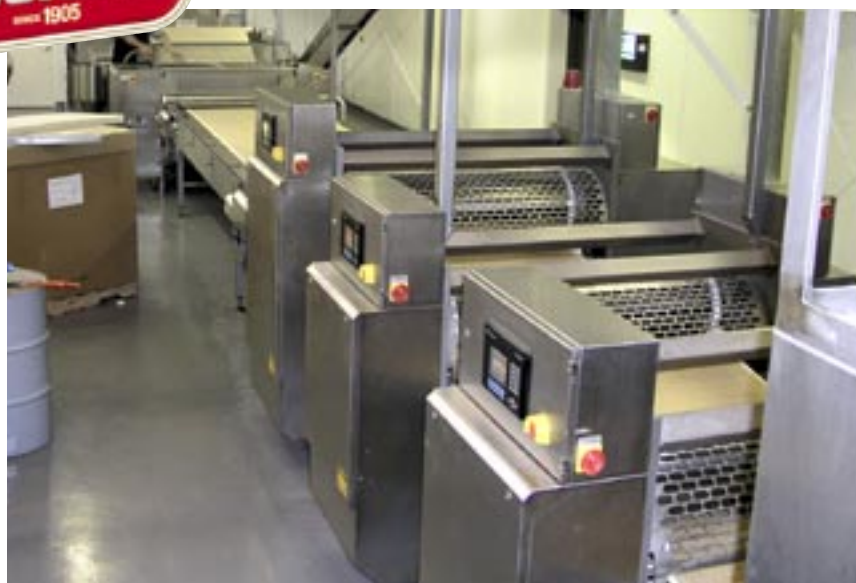
► The straight-line 3-stage reducing system (pictured) used for sandwich crackers fits neatly into the plant’s third production bay because of the small footprint vertical laminator and mezzanine-level mixing area.
