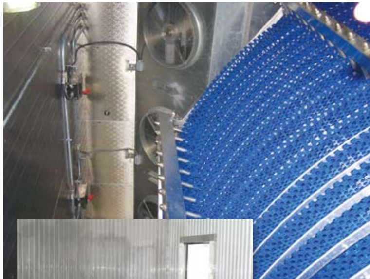
▲ PLC-controlled air temperature, air velocity (fan speed) and cooling/freezing time (belt speed) insure uniform quality cheesecakes, while the fully welded, 10-gauge stainless steel floors (inset) improve sanitation and cleaning in the spiral coolers and blast freezers.
