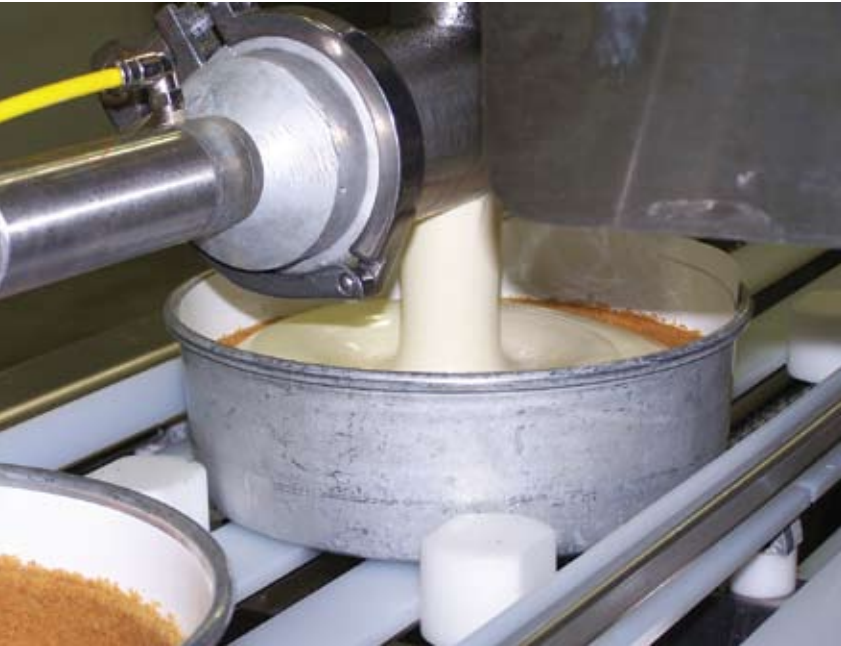
▲ This batter depositor uses a 3-in. feed pipe and depositing head to provide gentle product handling while maintaining ingredient integrity and quality.
