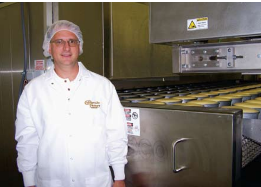
▼ Robert Michalski, plant manager, views the consistent color and overall appearance of freshly baked cheesecakes as they exit the 110-ft indirect-fired impingement oven.
