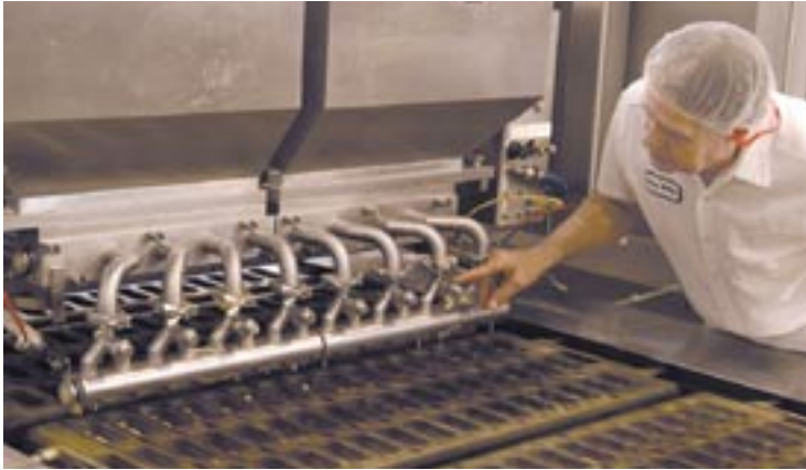
▲ Line operators perform most quality assurance tasks, including regularly taking weights at the depositor.
