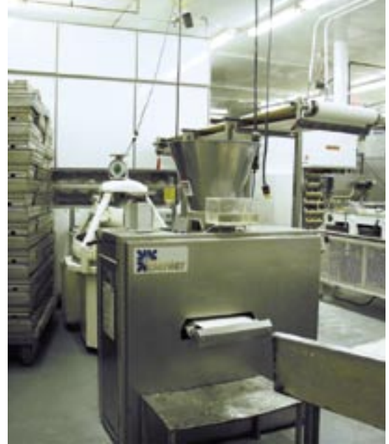
▲ A cross-grain depanner speeds preparation of bread loaves. The inmates operating this line are trained to make sure each dough piece is properly placed in the 5-strap pans.
