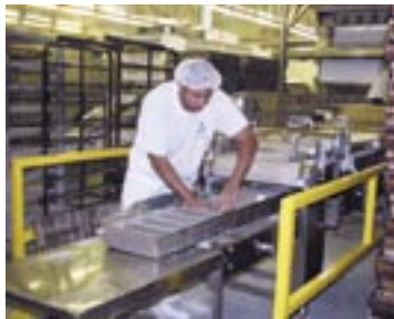
▲ A cross-grain depanner speeds preparation of bread loaves. The inmates operating this line are trained to make sure each dough piece is properly placed in the 5-strap pans.
