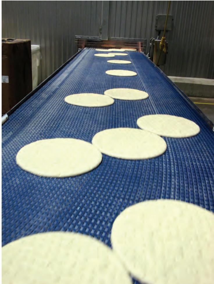
Par-baked pizza crusts travel from the oven along a conveyor into the bakery's blast freezer.
