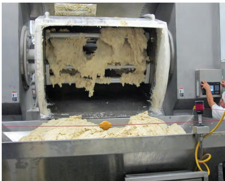
An operator dumps pizza dough from a 2,400-lb horizontal mixer into the hopper of a dough pump.
