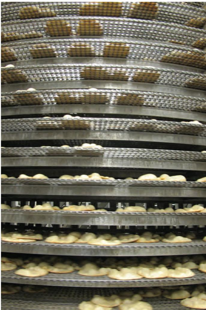
Kronos' freshly baked, 7-in. traditional pitas leave an oven (top) and head to one of two cooling systems (bottom) in a temperature-controlled area.
