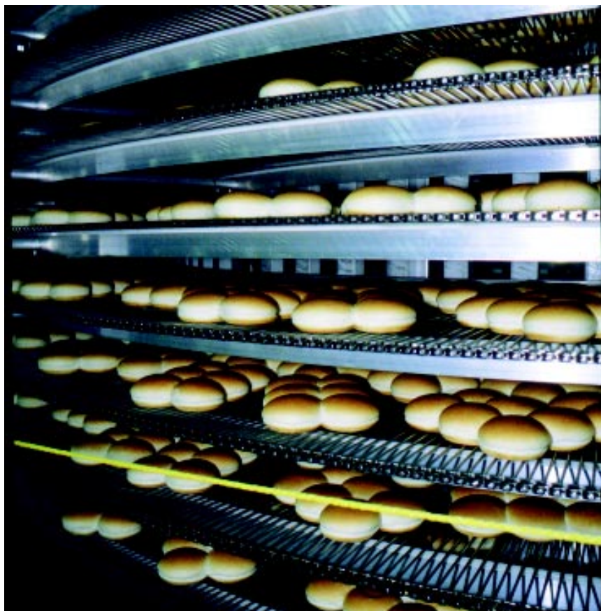
[Above] I.J. WHITE COOLING SPIRAL. Buns are uniformly cooled on a continuous belt.
