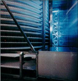
I.J. White's BF3000 spiral blast freezer, which St. James started up last month, already handles an estimated 3,000 lbs. of product per hour. The stainless steel, USDA-approved system and structure is 22 ft. wide by 28 feet long and 20 ft. deep. The model BF3000 — custom designed by I.J. White for St. James — features a new coil design that reduces defrost time. Moreover, the freezer has two infeed areas handling product from two separate production lines.
