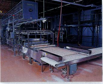
and return conveyors plus machinery for stacking and unstacking pans, we would have needed twice the space in our plant."
