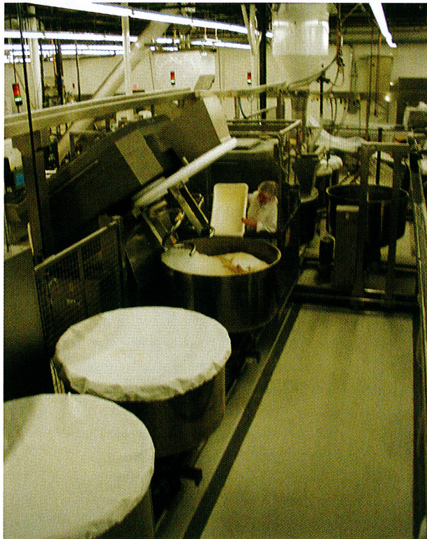
▲ In-line spiral mixers put doughs through mixing, kneading and resting stages. Multiple bowls mean maximum formula flexibility.
