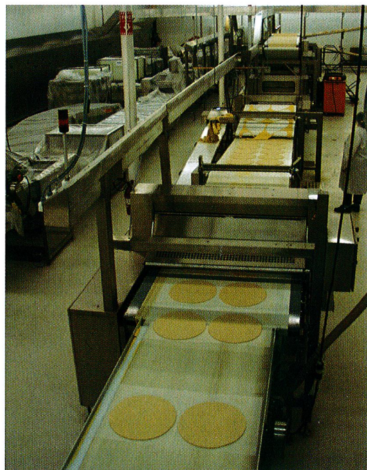
► Supplied by a single lamination line, the parallel makeup systems produce flat products [right] and rolled items [left]. Changeover is nearly instantaneous.
