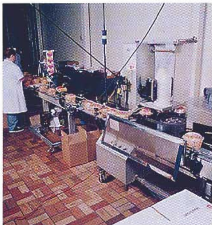
Tub cartons manually filled with sugar wafers supplement Voortman's bulk Cookie Hut line and consumer-size packages.
