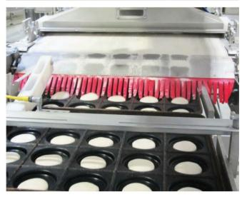
Top: A system accurately places the exact amount of sesame seeds atop 5-in. buns on the high-speed line. Middle: Dough pieces travel through rounder bars. Bottom: Panned dough pieces head to the bun line's proofer.
