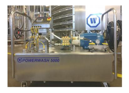
The POWERWASH® 5000 is a portable high-pressure washing system engineered to meet today's demanding requirements for improved sanitation in food processing plants. In one compact, all stainless steel system, the POWERWASH® 5000 ensures optimal hygiene with three complete wash cycles: Foam, Rinse, and Sanitize.
