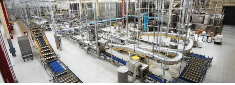
Bread dough pieces go through two side-by-side moulding stations before traveling in pans to the conveyorized proofer. production even while they're visiting other facilities.
