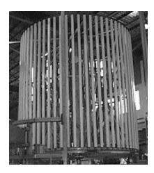
1. Only with the system turned "OFF and locked out, inspect the surface of the Wearstrips. Rub your hands on the surface, if your hand feels sticky, gritty, gummy or just dirty, then it is time to clean.
